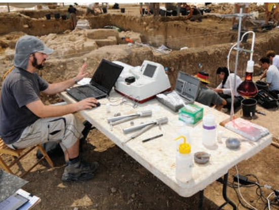
A portable spectrometer allows researchers to get a fuller picture of their samples during a dig.
